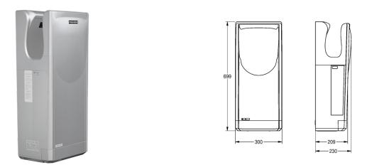
High Speed "Hands-in" hand dryer for wall mounting, antibacterial ABS plastic, colour silver, drying time 7-10 seconds, hygienic thanks to non-contact opto-electronically controlled release and integrated HEPA filter, adjustable air speed, optionally warm or cold air, auto shutdown after 25 seconds, water tank and discharge can be cleaned separately, protection class IPX4. Cable and plug not included in scope of delivery.
